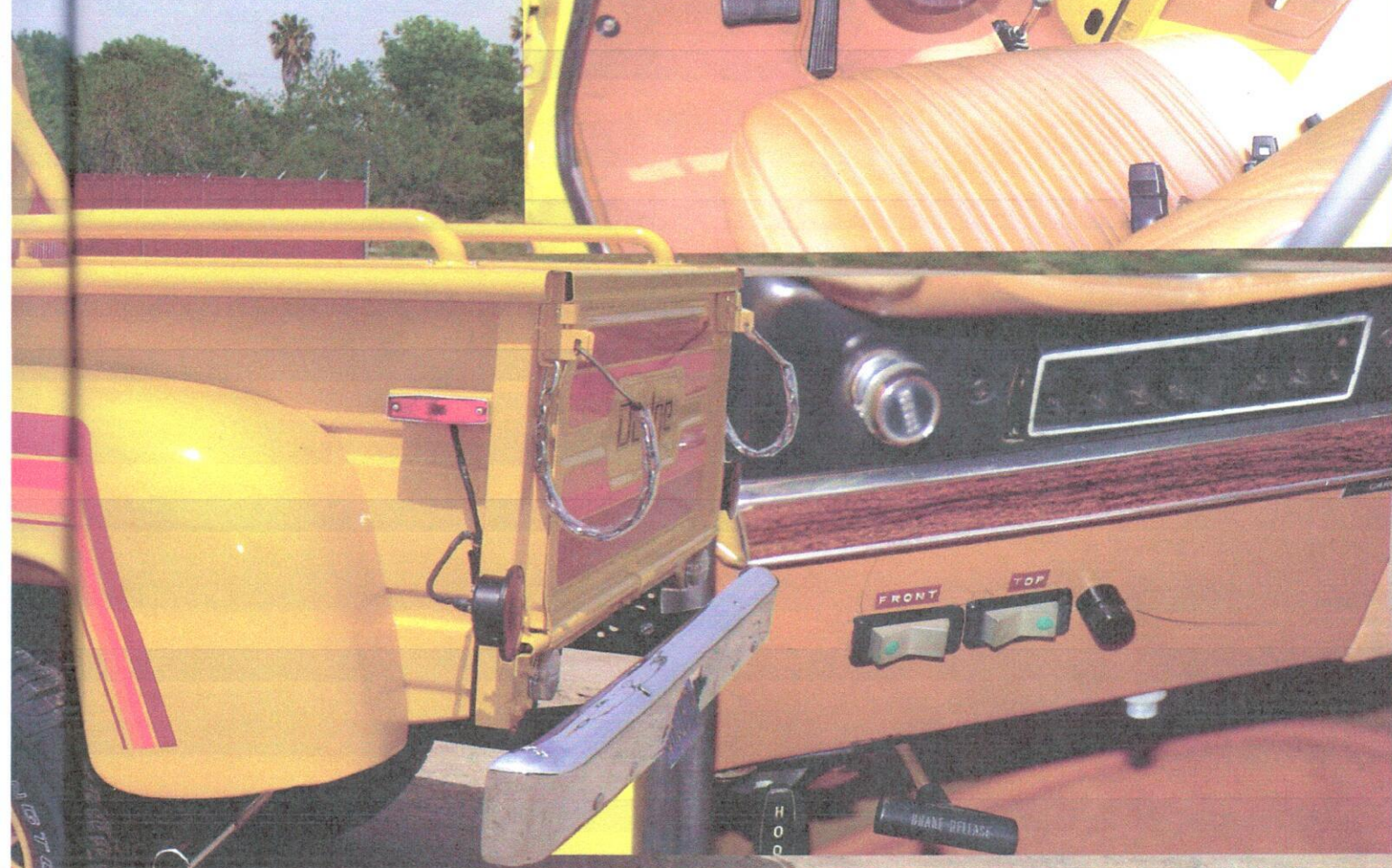
TO THE LEFT OF THE DASH YOU'LL FIND THE TOGGLE SWITCHES FOR THE BLINDING CIBIE OFF-ROAD LIGHTS THAT CAME STANDARD ON THE TOP HAND MODELS. AS CRUDE AS THIS INSTALLATION LOOKS BY TODAY'S STANDARDS, IT WORKS, AND THIS IS HOW THESE TRUCKS WERE MADE.
