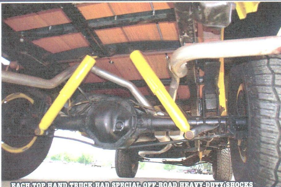
EACH TOP HAND TRUCK HAD SPECIAL OFF-ROAD HEAVY-DUTY SHOCKS INSTALLED BY HICKEY ENTERPRISES, AND ALL OF THESE TRUCKS CAME WITH SWAY BARS FRONT AND REAR.
